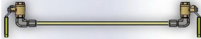
1.4.1 Sight Tube examples with isolating valves
